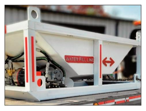
The WD300 consists of a 300 gallon hopper with in-tank mixers. The slurry pump is powered by a hydraulic motor that transfers slurry through a spray wand.
