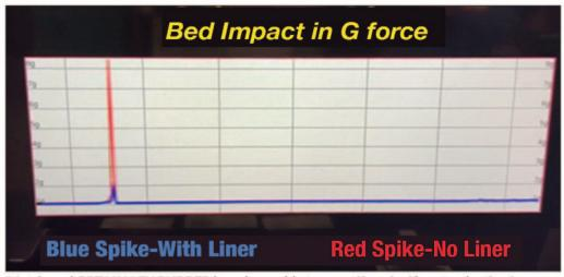
Matrix and GRT-VALLEY RUBBER have been able to quantify a significant reduction in "energy events" when using GRT-VALLEY RUBBER rubber-based solution compared with a steel truck bed
