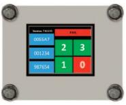
The Enhanced Status Screen (ESS) provides a quick visual report, showing if your system drivers and locators are working properly. ESS decreases the time required to trouble-shoot a system issue without the use of a laptop or other machine control interface tools.
