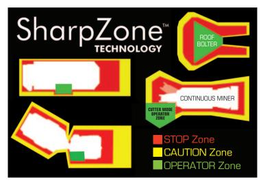
Unlike other prox systems, **Matrix IntelliZone** creates machine specific **straight-line and angled dynamic zones** which automatically change depending on the operational status of the equipment.
