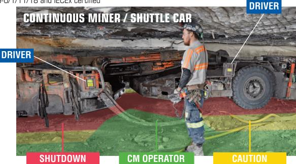
Immediately disables movement of equipment when locator detected in this zone.
