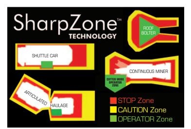
Unlike other prox systems, **Matrix IntelliZone** creates machine specific straight-line and angled dynamic zones which automatically change depending on the operational status of the equipment.
